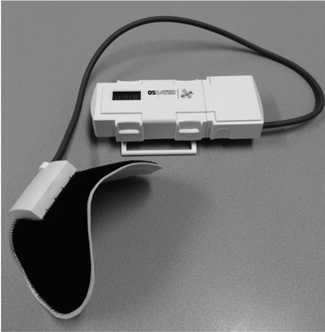
Figure 2. The PEMF bone growth stimulator consisting of a battery-powered signal processor and a flexible flat coil.
